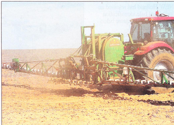
□ A boomsprayer with a weedseeker attached being used to spot spray weeds.
